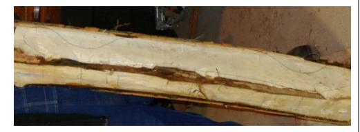
The selected timer is roughed to shape and layout lines are added with a pencil.
