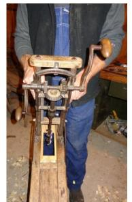
After the layout, the holes are drilled before the shaping begins. Only animal and human power allowed. Once the holes are drilled the shaping work begins. All done with hand tools that can be constructed in the local communities.
