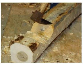
There are many ways to approach the removal of the wood, such as saw kerfs and chisels, but in the places that Tillers goes to such a Mozambigue or Uganda, a farmer may only have a machete or hoe. It was noted they can do impressive work with only basic tools like a machete or ax. After the roughing process the finer hand tools are used to achieve the final shape.
