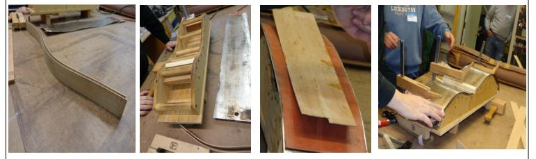
Another bending tool Doug uses is an Ibex bending iron. It elliptical shape gives it more bending surfaces than a typical heated pipe. The wood side strips are typically resawn, rough sanded, hand planed and scraped to 1/8" thick or less. Distilled water is used during bending to prevent chemical staining from sanding grit and minerals. Wetting the bands has a technique as well. Too much water causing cupping, however more water is needed at
