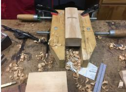
center section to make a space for the plane iron and wedge. Truth is that Chuck makes it look simple, but there are precise angles to be cut and proper gap spacing for optimal performance.
