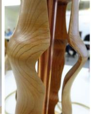
Don Squires brought in an unusual lamp. It started as a single piece of wood cut on the band saw into four pieces. The four pieces are shaped on the band saw, turned inside out and glued back together, leaving a hollow core. The new piece of wood is then turned on a lathe creating the four ribbon sides of the lamp. Don also brought in a bowl he turned from a unique piece of yellow
